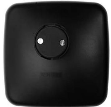
Part Number: M2382CE Dimensions: 193 x 193mm Fits mirror arms: 16-28mm
